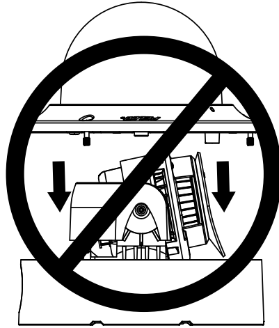
Figure 13. Incorrect Dome Cover Attachment Method
